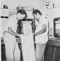
MODERN ELECTRONIC vapor fractometers analyze light refinery streams for the individual hydrocarbon components. Left is Bill Sanders, chemist, and Max Tromp, analyst.
